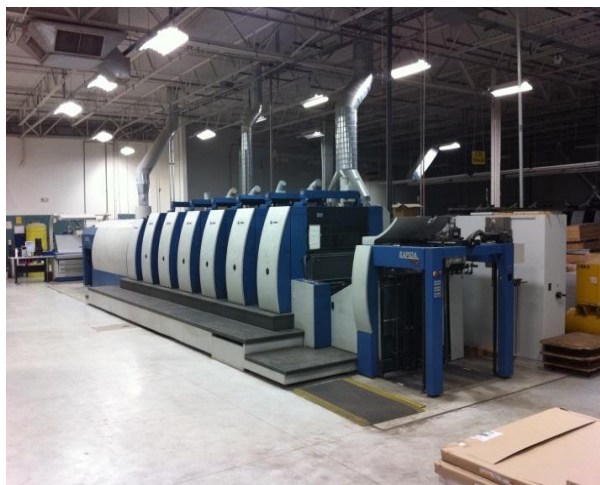
KBA Rapida 105 29' x 41' format 6/C; UV Interstation & IR dryers; 18,000sph; delivery and feeder Commercial Lithography Press. Next Genius 52 UV Waterless Press for Lenticular & Plastic 24Pt
