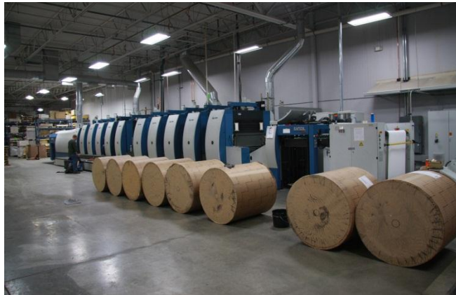
KBA Rapida 105 10/c Perfector; UV Dryers interstation 29" x 41" Format: 5/5 13,000sph; Mabec sheeter for roll fed to compete with the Web Press's but have the quality of offset.
